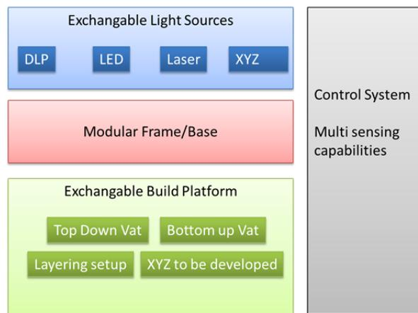
Fig. 1: Modular research platform for additive manufacturing by stereolithography
